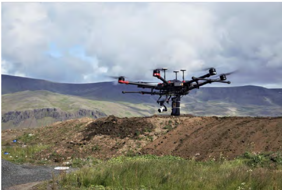
Figure 6. Drone equipped with a laser methane sensor mapping the methane concentration at the Álfarnes landfill outside Reykjavik, Iceland 31 .
